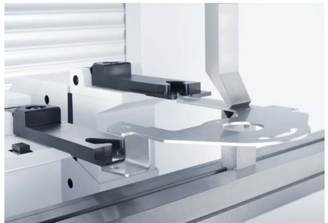
Flexible production thanks to the 6-axis backgauge.
