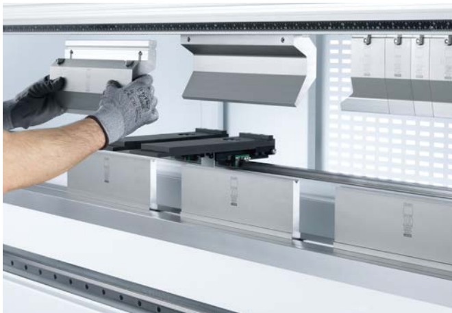
Easy loading of tools from below thanks to Safety Click.
